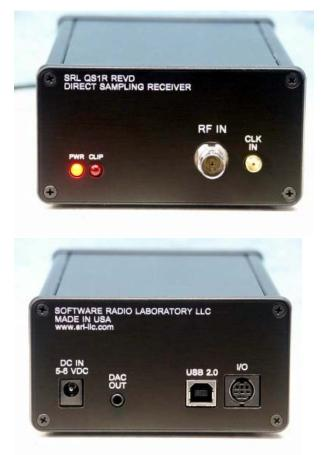
The QS1R receiver, when used with the Afreet Skimmer Server software, can provide CW decoding of up to 192 kHz of each of seven bands simultaneously, and provide all decoded callsigns heard in the form of telnet spots. Full specifications are at <a href="http://www.srl-llc.com/files/qs1r">http://www.srl-llc.com/files/qs1r</a> revd specs.pdf.
