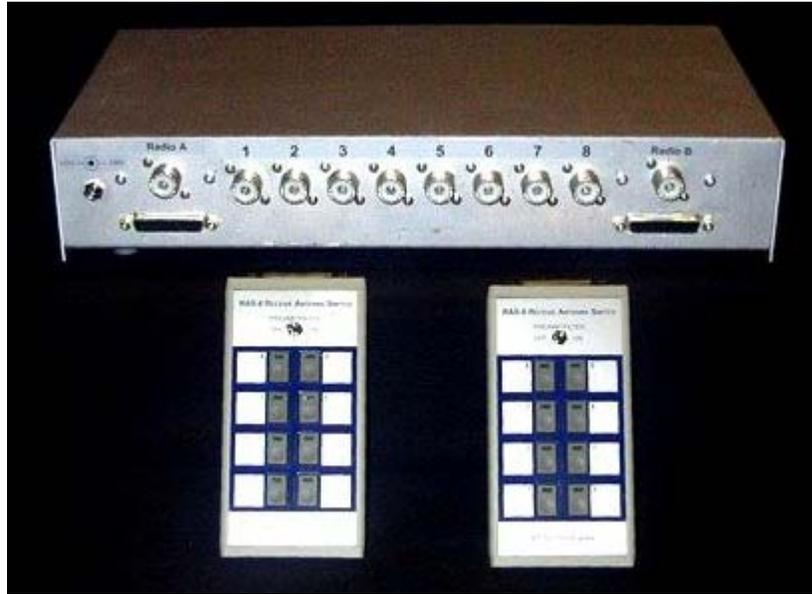
The RAS-8x2 provides flexible switching for your receiving antennas. Eight antennas can be routed to either of two radios, selected with remote keypads that fit easily into your shack. Preamp/filters for each radio provide 12 dB or more gain and filtering for 1.8-4.5 MHz (160M & 80M). When the preamps are OFF, the filters also are bypassed and the unit may be used on any frequency <math><0.5\text{ MHz}</math> to 30 MHz.
